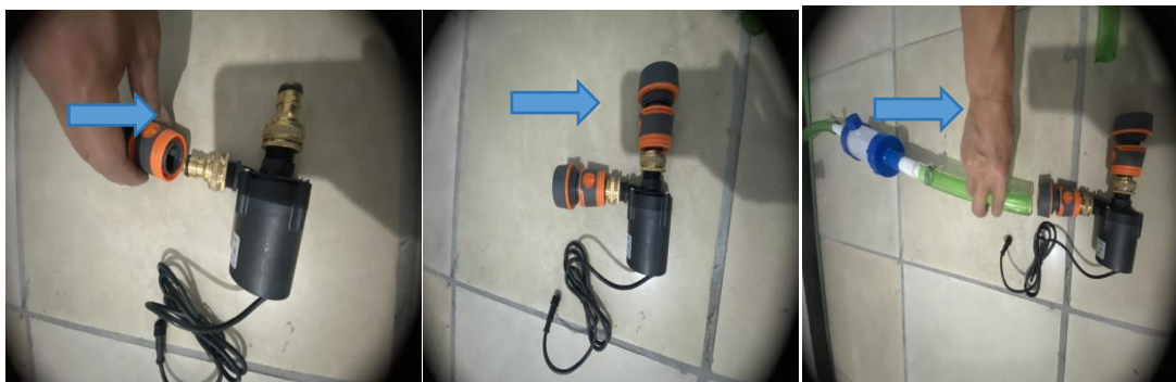
Screw the quick connector female to the circulation water inlet
