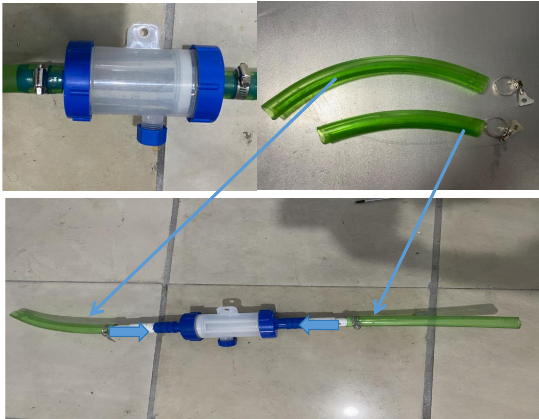
4.2: Connect the circulation pump and filter assembly
